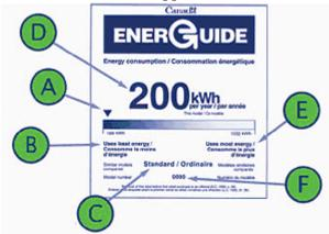
**A** - The energy consumption arrow just above the shaded bar scale shows how this model compares with the lowest-rated (to the left) and the highest-rated (to the right) model of the same type.
